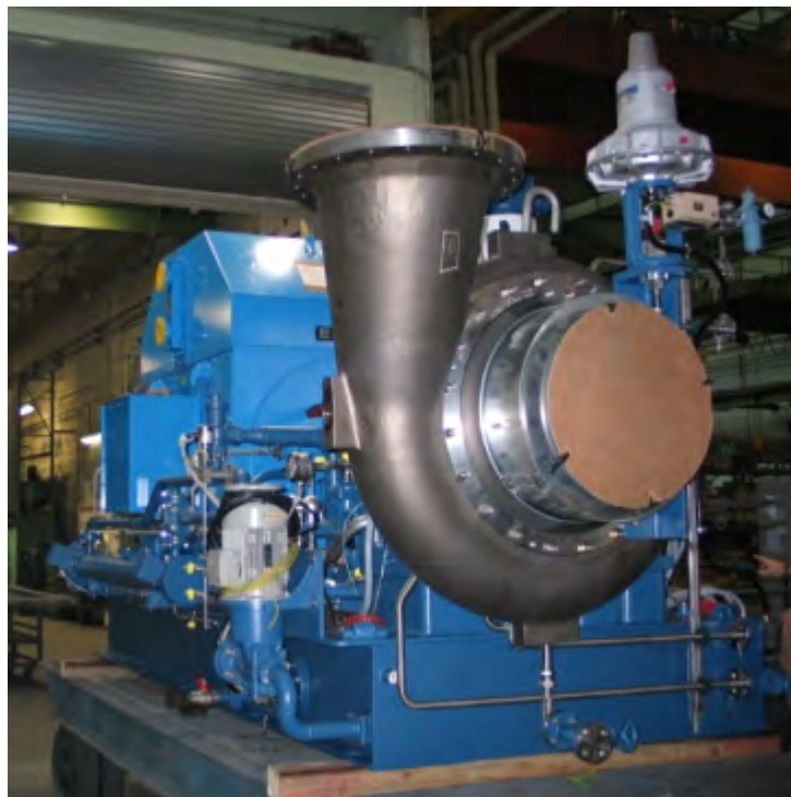
Mechanischer Brüdenverdichter (Turbokompressor) Mechanical vapour compressor (turbo compressor)
