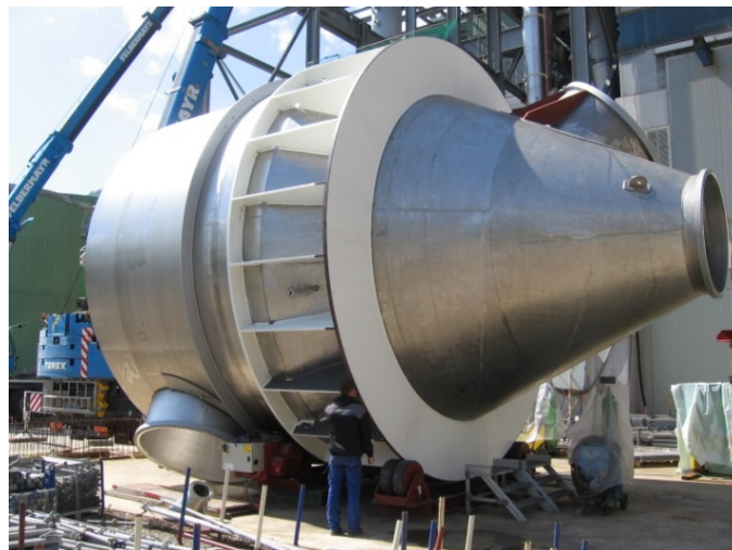
Site fabrication and mounting (Austria) Evaporation crystallizer Ø 6.400 mm, overall length 18.700 mm, 56 t, 1.4562
