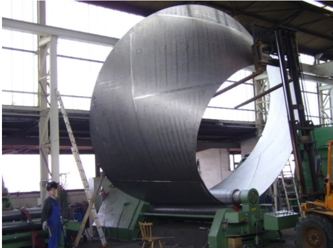
Site fabrication and mounting (Austria) Evaporation crystallizer Ø 6.400 mm, overall length 18.700 mm, 56 t, 1.4562
