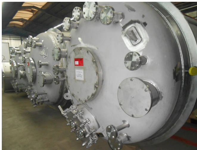
Stirring tank Ø 2.400 mm, 1.4571
