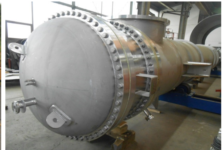
Manufacturing of pre heaters for evaporation crystallization Ø 800 mm - Ø 1.300 mm, overall length 11.700 mm, weight 8,8 - 21,8 t, Aluminium bronze
