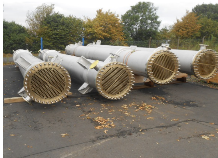
Manufacturing of pre heaters for evaporation crystallization Ø 800 mm - Ø 1.300 mm, overall length 11.700 mm, weight 8,8 - 21,8 t, Aluminium bronze
