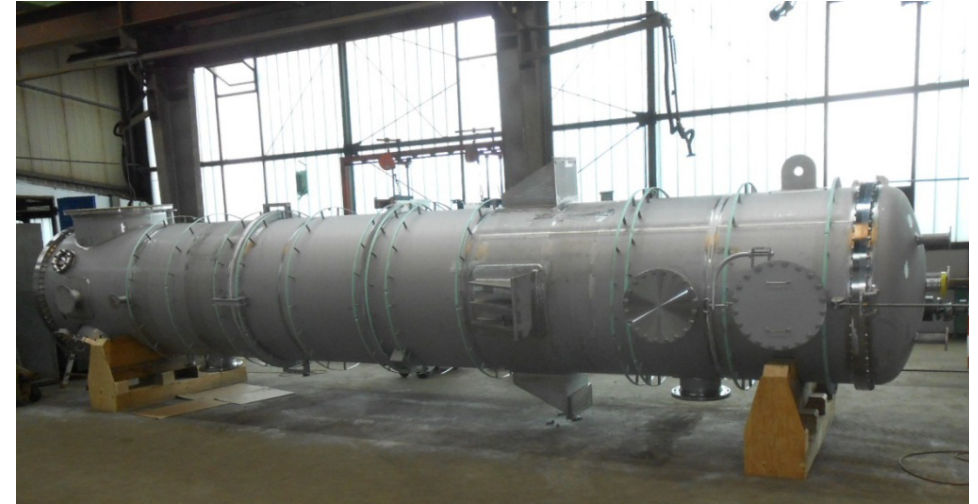
Plume-condensator Ø 1.800 mm, 1.4541
