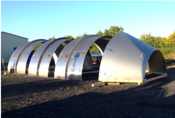
Site fabrication and mounting (Russia) Evaporating crystallizer Ø 5.400 mm, overall length 21.800 mm, 40 t, 1.4562
