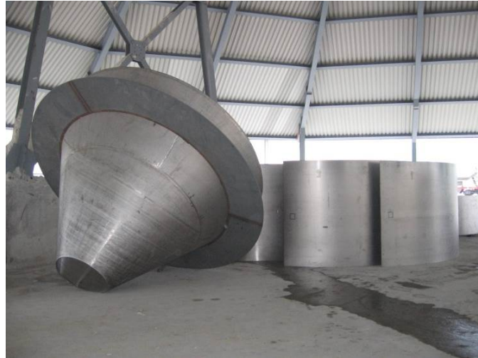
Site fabrication and mounting (Austria) Evaporation crystallizer Ø 6.400 mm, overall length 18.700 mm, 56 t, 1.4562
