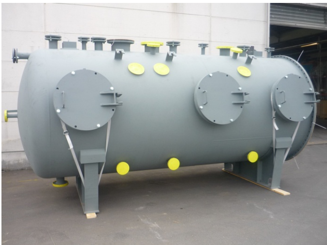
Crystallizer part Ø 1.800 mm, steel/rubber lined
