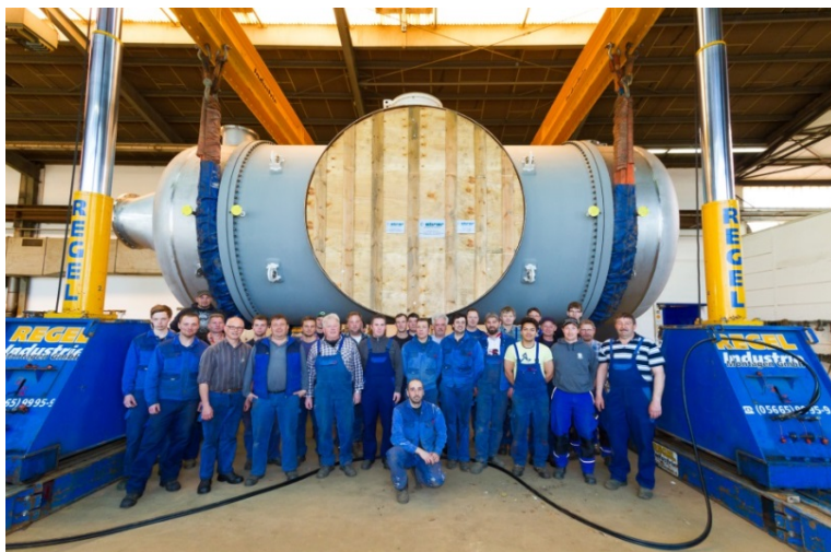
Manufacturing and mounting (Netherlands) Sea water condenser Ø 3.650 mm, overall length 10.000 mm, 40 t, 1.4462/P355GH
