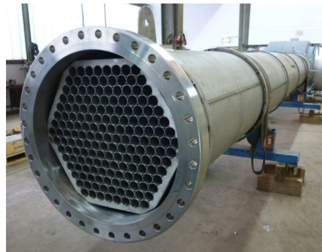
Flow modifier Ø 950 mm, 1.4404
