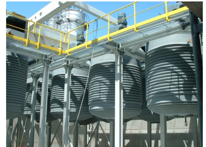
Manufacturing and mouting of agitator tanks incl. EMSR-Technology (Germany) Ø 2.200 mm - Ø 3.000 mm, overall length 5.700 mm, weight 7 - 11,6 t, Steel
