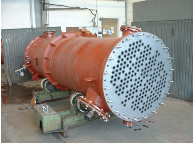
Heat exchanger in various materials such as Monel, Titanium, Graphite
