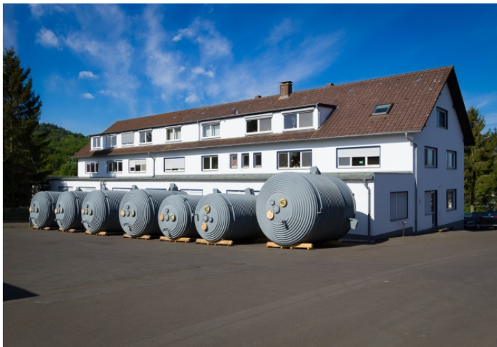
Manufacturing and mouting of agitator tanks incl. EMSR-Technology (Germany) Ø 2.200 mm - Ø 3.000 mm, overall length 5.700 mm, weight 7 - 11,6 t, Steel
