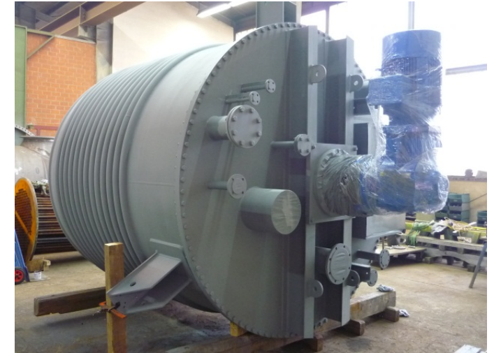
Manufacturing and mouting of agitator tanks incl. EMSR-Technology (Germany) Ø 2.200 mm - Ø 3.000 mm, overall length 5.700 mm, weight 7 - 11,6 t, Steel
