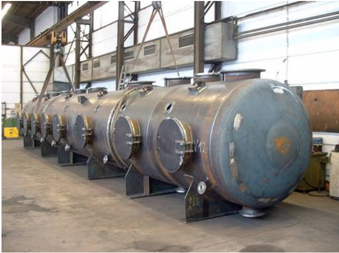
Flash evaporator Ø 3.500 mm, steel/rubber lined
