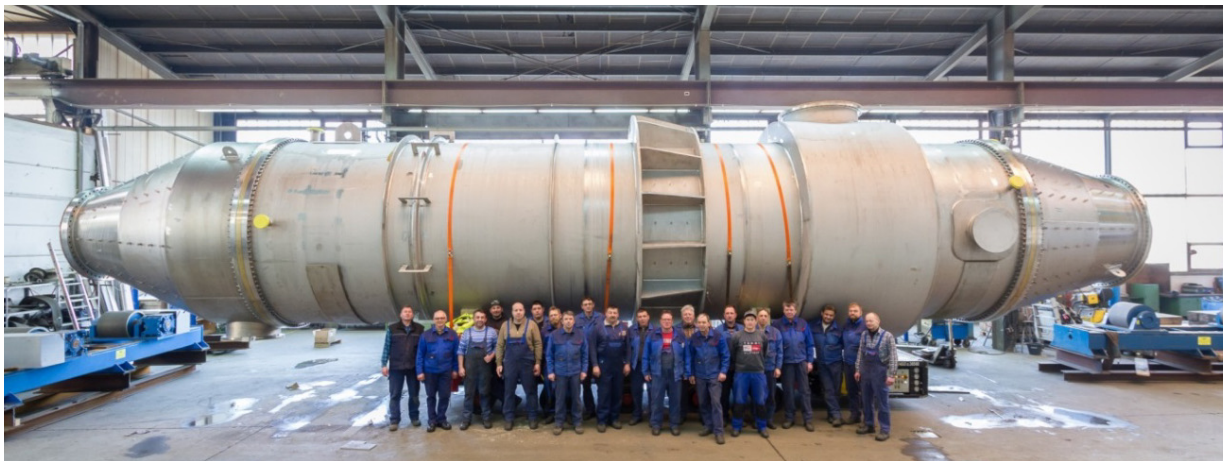
Heat exchanger Ø 3.150 mm, tube length 9.000 mm, 113 t
