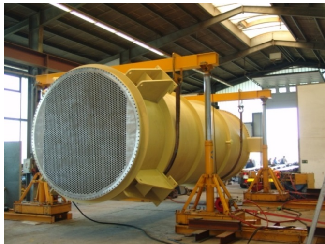
Heat exchanger in various materials such as Monel, Titanium, Graphite
