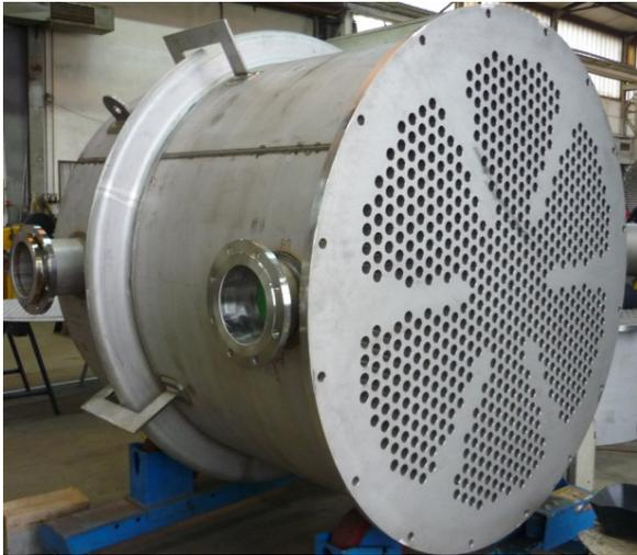
**Oleumkondensator** Ø 1.650 mm, 1.4571
