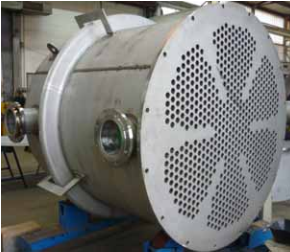
Oleumkondensator Ø 1.650 mm, 1.4571
