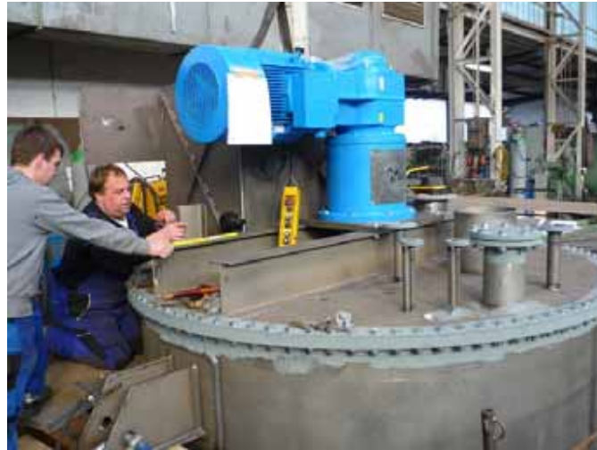
Manufacturing and mouting of agitator tanks incl. EMSR-Technology (Germany) Ø 2.200 mm - Ø 3.000 mm, overall length 5.700 mm, weight 7 - 11,6 t, Steel
