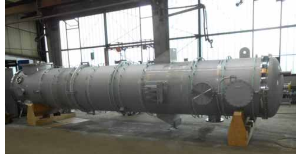
Plume-condensator Ø 1.800 mm, 1.4541
