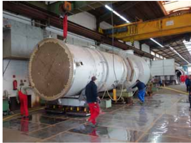
Heat exchanger Ø 3.100 mm, overall length 17.640 mm, weight 113 t A special transport on air cushions was necessary
