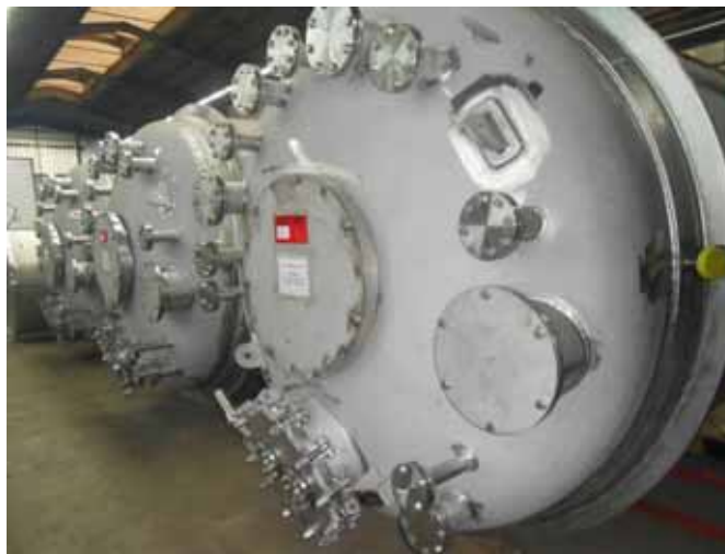
Stirring tank Ø 2.400 mm, 1.4571
