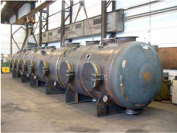
Flash evaporator Ø 3.500 mm, steel/rubber lined
