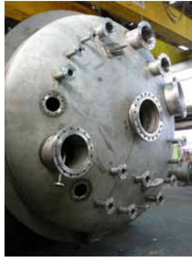
Reactor Ø 3.500 mm, 1.4539
