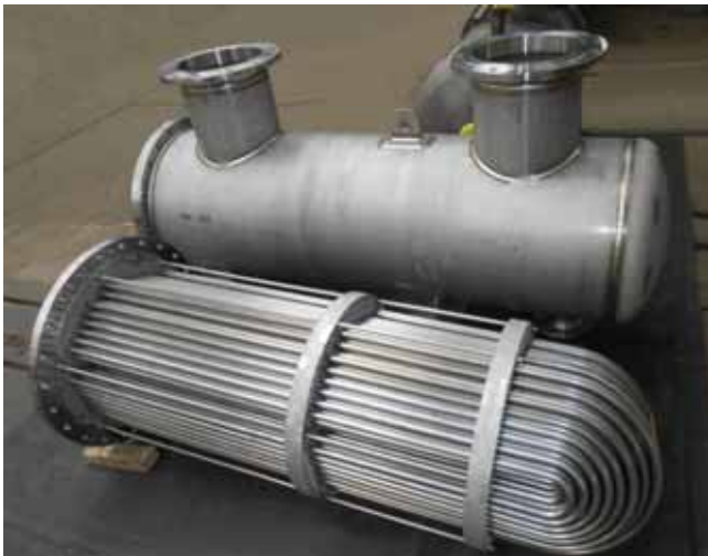
Condensator with pullable bundle Ø 610 mm, 1.4571
