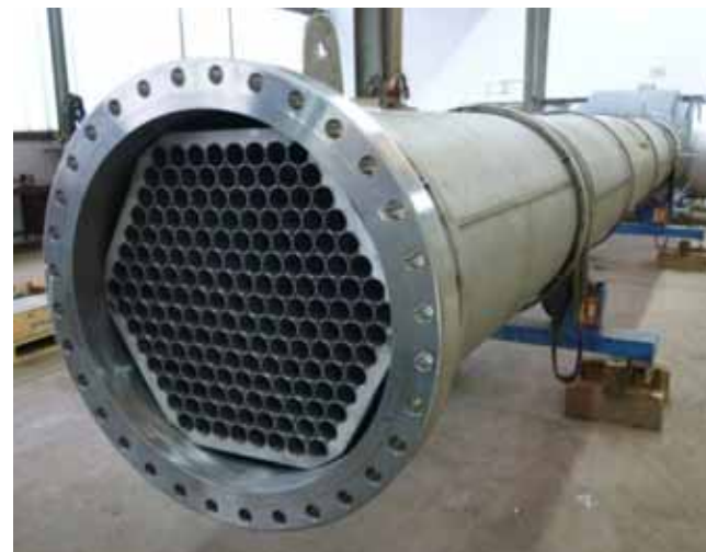
Flow modifier Ø 950 mm, 1.4404
