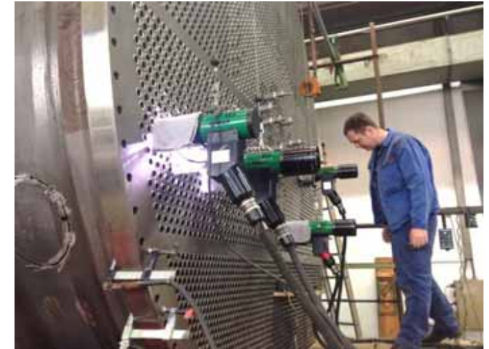
Manufacturing and mounting (Netherlands) Sea water condenser Ø 3.650 mm, overall length 10.000 mm, 40 t, 1.4462/P355GH
