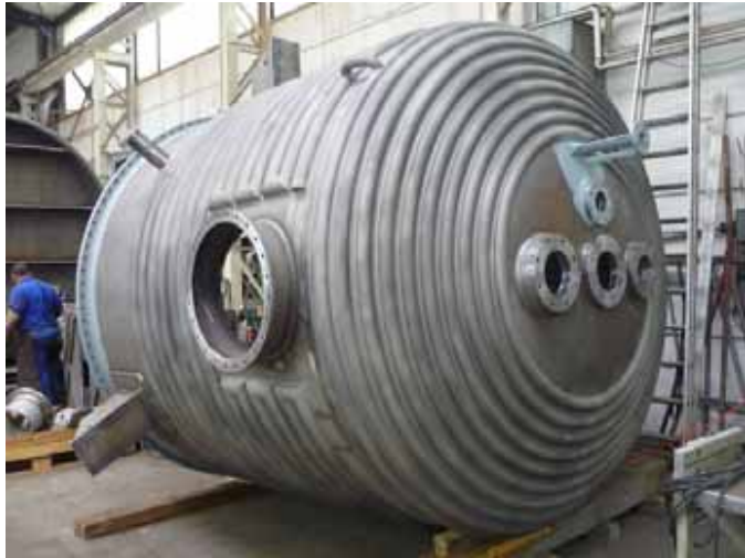
Manufacturing and mouting of agitator tanks incl. EMSR-Technology (Germany) Ø 2.200 mm - Ø 3.000 mm, overall length 5.700 mm, weight 7 - 11,6 t, Steel
