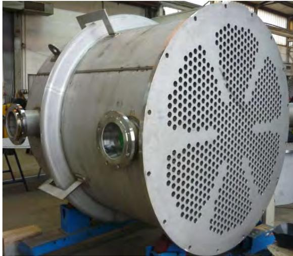
**Oleumkondensator** Ø 1.650 mm, 1.4571
